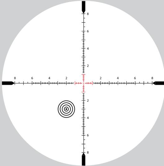
*Use 3 mil to compensate a 54 inch bullet drop for a target at 500 yards, 2 mil wind correction for 15 mph wind from right to left.*
